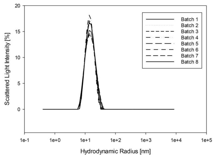
Fig. 3. Dynamic light scattering of Octanorm (overlay of eight batches); samples diluted 1:5 in 0.9% sodium chloride. Triplicate measurements of each Octanorm batch were performed and the results represent the respective arithmetic mean.
